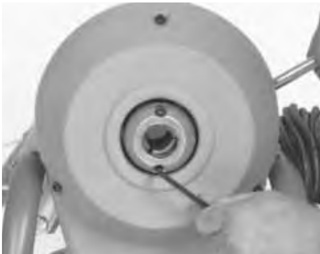
Figure 12 – Replacing Clutch Jaws
